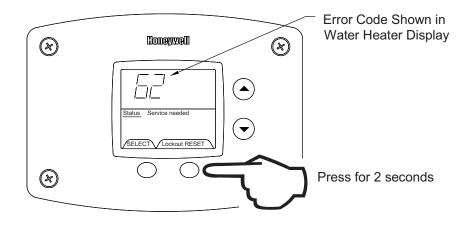
All other error codes will put the water heater into a "Hard Lockout" condition, in which the water heater will not operate and cannot be reset in the "User Mode". To reset a hard lockout, first enter the "Service Mode" described earlier by pressing both the "Temperature Up" and "Select Buttons" at the same time for 3 seconds. Then press the lower right button under "Lockout Reset" in the water heater display and hold for 3 seconds.
